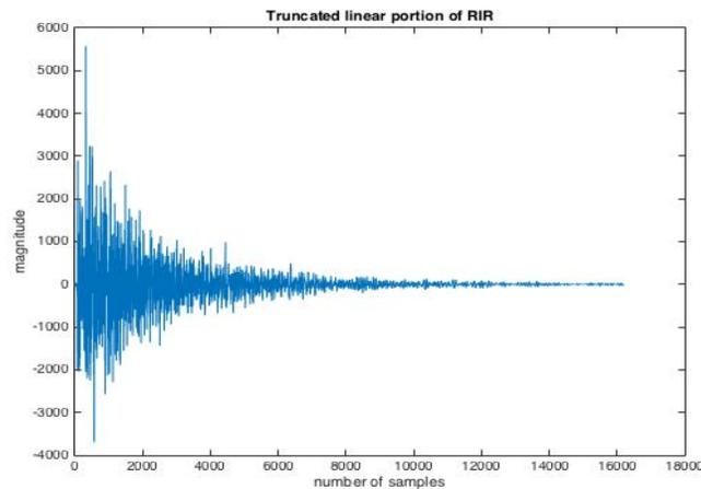
Figure 5: The windowed impulse response to approximate the linear portion of the large rooms' acoustic response. The entire system operated on a sampling rate of 16 kHz.
