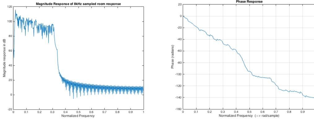
Figure 8: The magnitude and phase responses of the IR approximated in Figures 7. The actual value of the magnitude response was purely qualitative, as it was a function of the magnitude of the recorded input. The frequency axis was normalized to half of the sampling frequency; therefore the frequency 1 corresponded to a frequency of 8 kHz .
