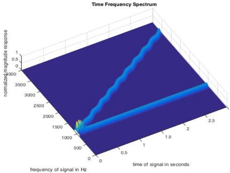
Figure 3: The joint Time/Frequency spectrum of the input signal corresponding to (10). The image shows clearly the desired response of both the modulated chirp and cosine signals.
