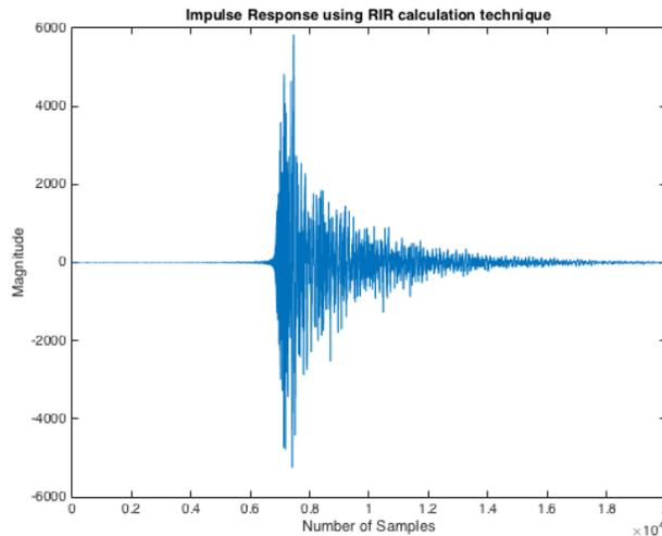
Figure 7: The windowed impulse response to approximate the linear portion of the small rooms' acoustic response. The entire system operated on a sampling rate of 16 kHz.
