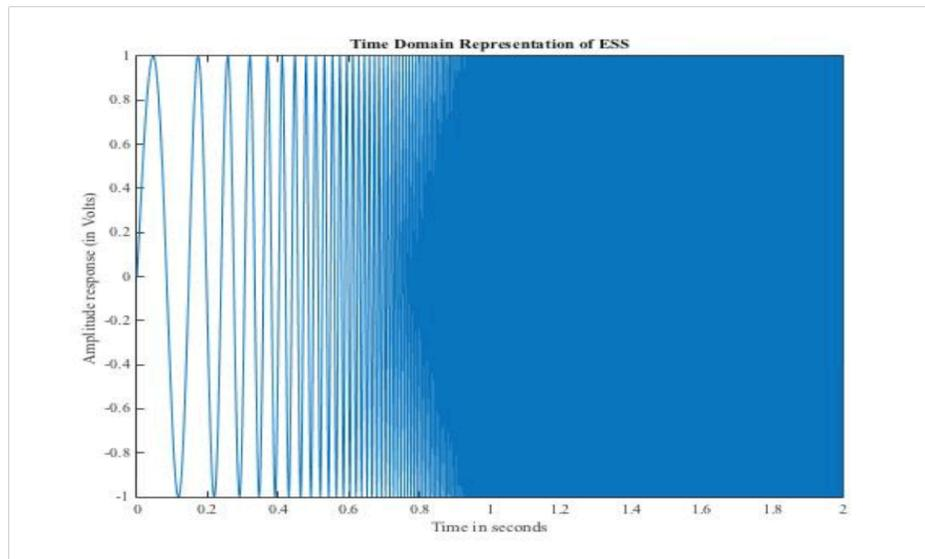
Figure 1: A 2 second ESS wave sampled at 44.1 kHz swept from 5 Hz to 15 kHz.
