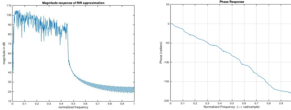
Figure 6: The magnitude and phase responses of the IR approximated in Figures 4 and 5. The magnitude was set to an arbitrary scale, and thus was qualitative. The frequency axis was normalized to half of the sampling frequency; therefore the frequency 1 corresponded to a frequency of 8 kHz .
